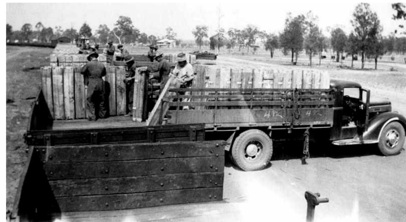
Loading the munitions' onto the train for shipment to the pacific theatre. Note: the wooden packaging was ironbark for transport to the tropics as the US packaging as it arrived in Australia was cardboard tubes.
